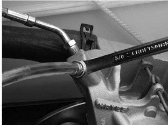
10. Torque the bleeder screw to 8-11 ft.-lb. (11-15Nm).
