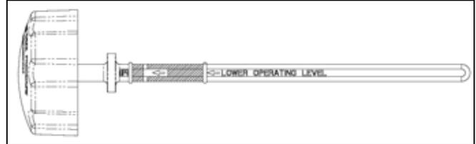
9. If the oil level is high, the excess oil MUST be removed from the storage tank. Again, remove excess oil from the tank in 2 oz. increments.
