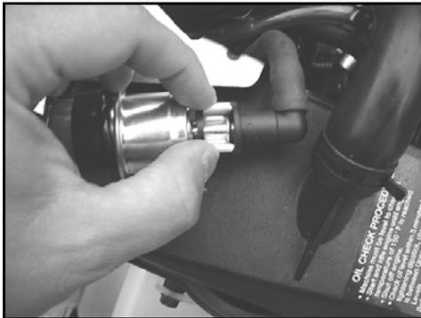
1. Slide the Posi-Lock connector onto the fitting past the flange until an audible “click” is heard.
