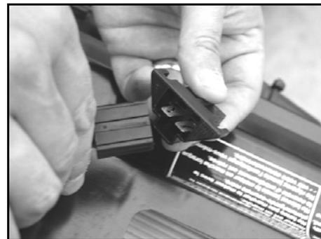
**NOTE: The ECU will remain powered as long as the jumper is installed. When finished, always remember to remove the jumper, and reconnect the ignition switch connector!**
