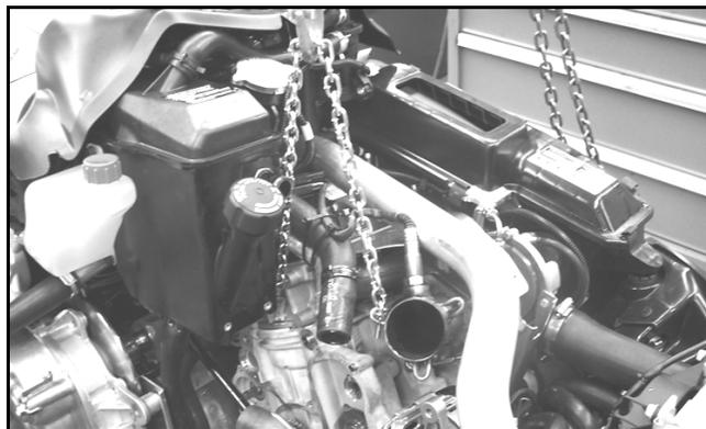
4. Slowly lift the hoist just enough to support the weight of the engine.
