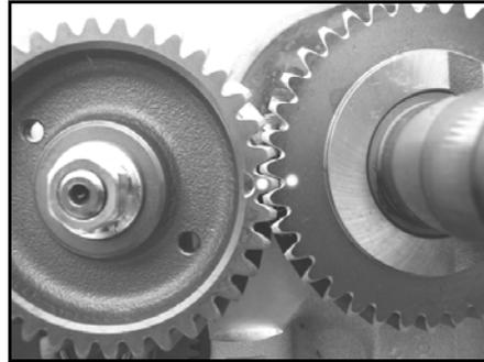
The pistons are at TDC when the set of SINGLE timing marks are aligned with each other, and the set of DOUBLE timing marks are aligned with the upper and lower crankcase parting line.
