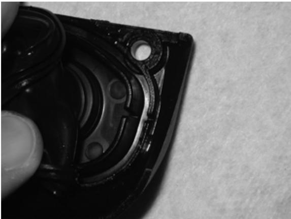
2. Remove the two T-15 Torx screws from the cover.
