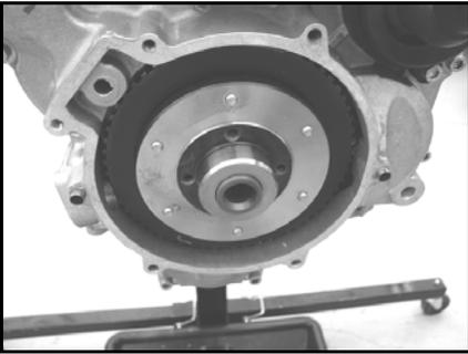
**NOTE: When the flywheel is properly seated on the locating pin, turning the flywheel will turn the crankshaft.**
