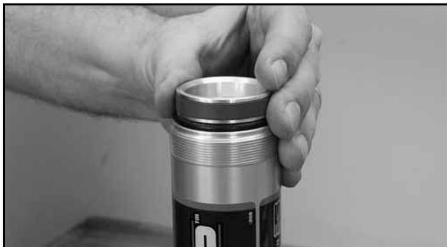
13. Using the IFP locator tool, slowly push the IFP down into the cylinder. The IFP is set to the correct position when the indicator knob makes contact with the shock body.
