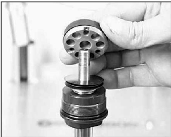
4. Place a new lock nut onto the shock rod. Torque the new lock nut to specification.
