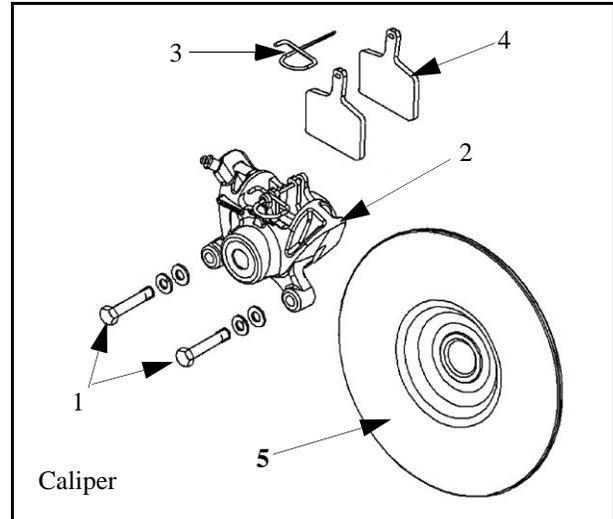
1. Remove the two caliper bolts that hold the caliper to the chaincase.
