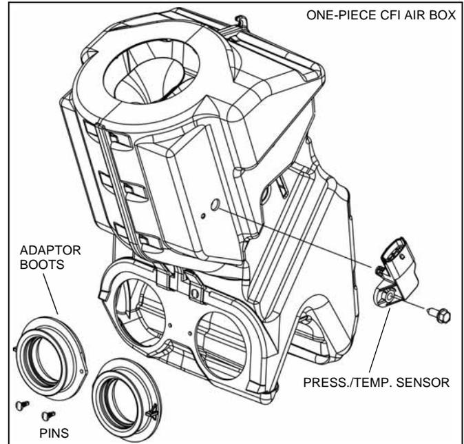
**NOTE:** All 2007 and some 2008 CFI models were manufactured with a two-piece airbox where an adapter plate was secured to the throttle body. The airbox then snapped into the adapter plate to make the airbox assembly.
