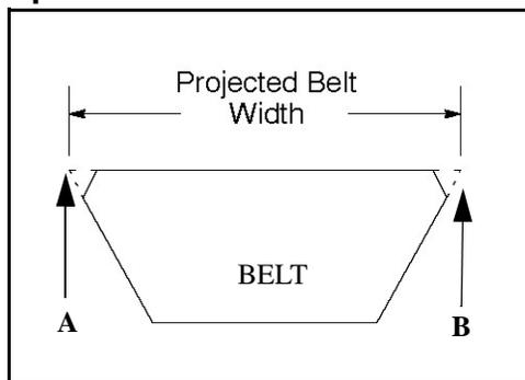
1. Measure the belt width and replace it if it is worn severely. Generally a belt should be replaced if the clutches can no longer be adjusted to provide the proper belt deflection.
