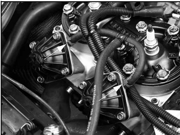
15. Remove the drive belt, driven and drive clutches. See Chapter 6.
