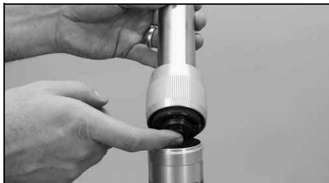
18. Slowly push the piston rod into the shock body until the cylinder head assembly bottoms on the cylinder counterbore. Slight up and down movement may be required to allow all air to pass through the piston assembly.
