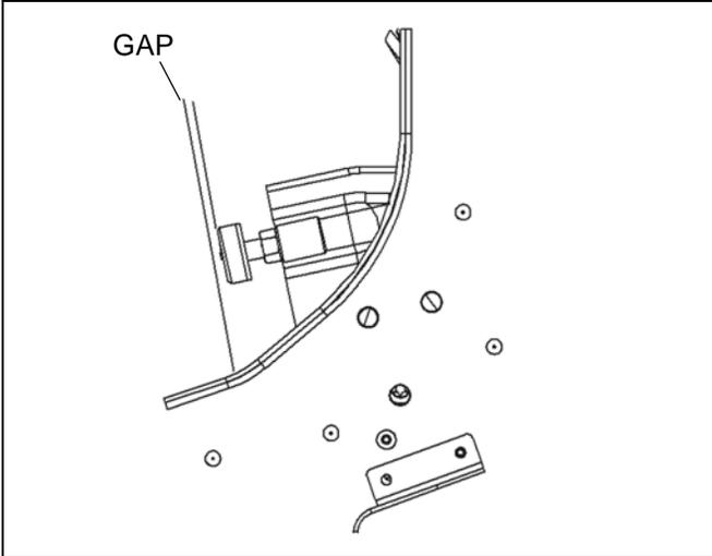
Set torque stop bumper gap to specification after aligning drive and driven clutches.
