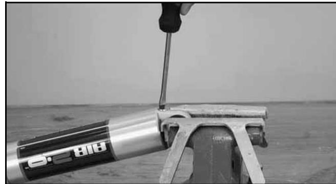
5. After all of the nitrogen gas has been allowed to escape from the shock, remove both pressure valve assemblies.
