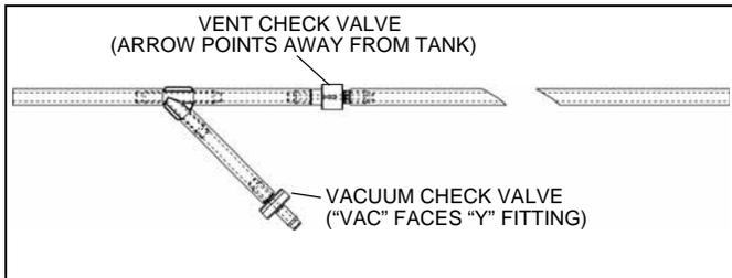
Some models feature a rollover check valve / vent / vacuum check valve assembly bonded to the inside of the fuel tank. The rollover check valve prevents fuel from escaping the tank in the event of a vehicle rollover.
