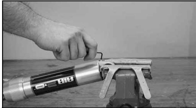
4. Using a flat-blade screwdriver, carefully loosen both pressure valve assemblies counter-clockwise two full rotations. Allow all of the nitrogen gas to fully escape past each pressure valve assembly o-ring.
