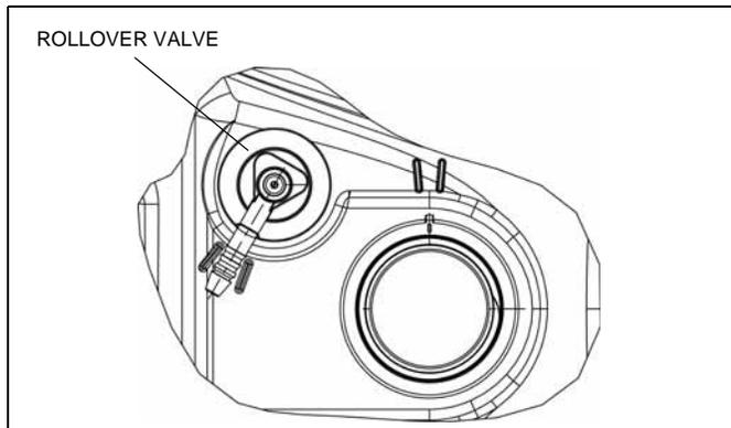
The rollover check valve is not serviceable. When inspecting the system, verify the hose is not kinked.
