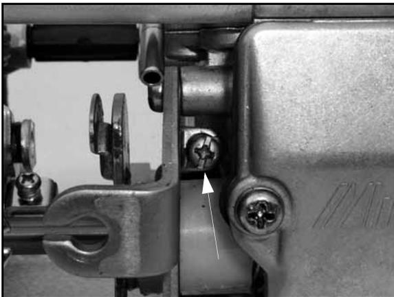
6. Once the PTO carburetor slide is flush, loosen the Phillips head screw, located under the top cover on the MAG carburetor.
