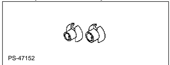
1. To disconnect a fuel hose from the fuel pump, or fuel rail, insert the tapered end of either the 5/16" or 3/8" tool into the female housing.
