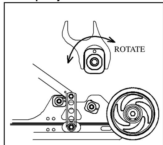
The front rear scissor stop (FRSS) controls the bump attitude of the rear suspension. As the front torque arm (FTA) hits the bump, it forces the rear scissor to collapse a predetermined amount, depending on the FRSS block position.
