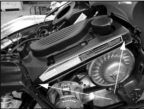
41. Install the Nylock nuts and two T40 Torx bolts to the front and the two T40 to the rear of the LH and RH chassis brace and install the braces.
