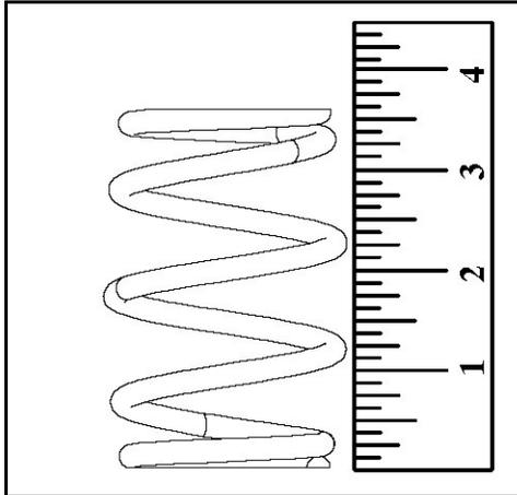
In addition to proper free length, the spring coils should be parallel to one another when placed on a flat surface. Distortion of the spring indicates stress fatigue. Replacement is required.
