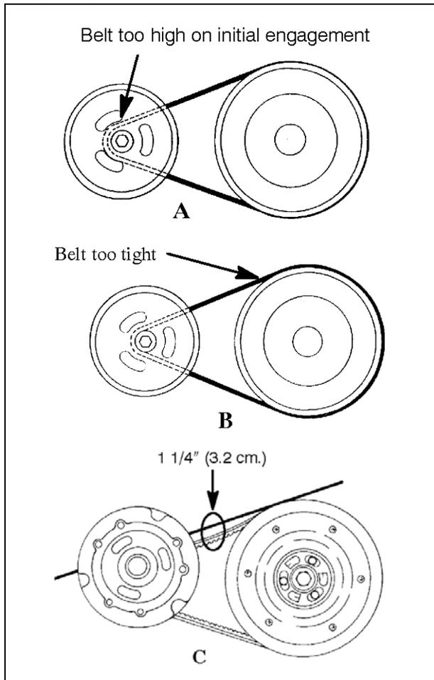
1. Measure the belt deflection with both clutches at rest and in their full neutral position.
