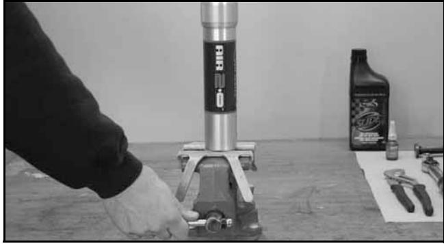
3. Remove both small bottom head screws from each pressure valve assemblies located at both ends of the shock.
