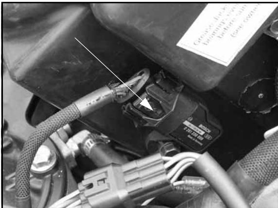
7. On CFI models, remove the return fuel line "P" holder located on the MAG side of the airbox.
