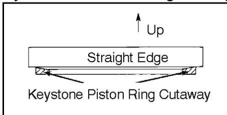
Piston rings are installed with marking or beveled side up.
