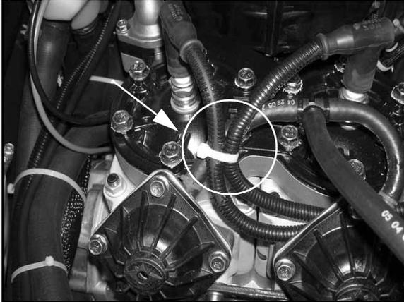
40. Install the electrical center/belt holder over the electrical center by aligning the rear buttons to the rear of the clutch cover and installing the two fasteners.
