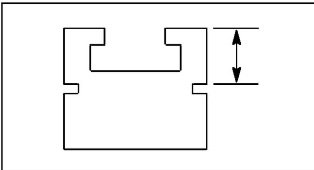
Replace sliders when wear exceeds notch. If sliders look “wavy” in appearance, check and adjust track tension or consider adding more bogie wheels.
