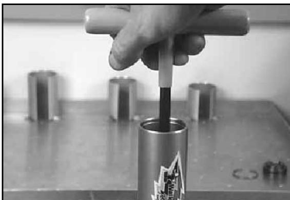
9. Remove the IFP from the reservoir with the IFP tool (PN PS-45908).
