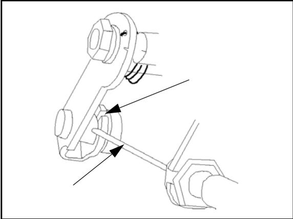
34. Remove the cable from the oil pump bracket.
