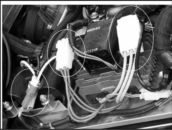
13. Disconnect the EV solenoid from the ECU harness.
