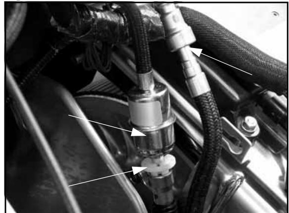
27. Secure the loose fuel lines out of the way for engine removal.
