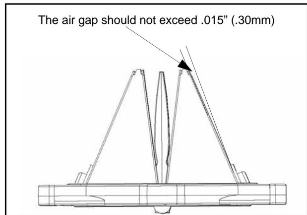
7. If damaged remove and replace the reeds on the reed cage.
