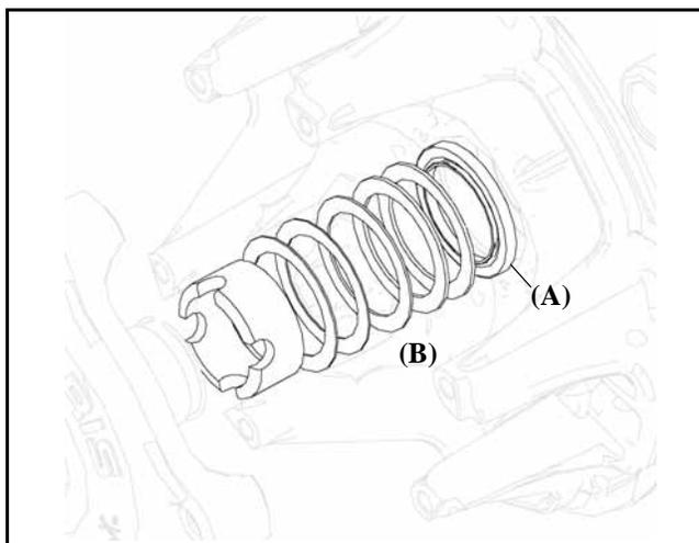
4. Install spider washer(s) and spider aligning the "X" with the moveable sheave's "X". Notice as the spider seat location is changed, the sheave marks made before disassembly no longer align (C). There are two ways to bring the sheave marks into alignment.
