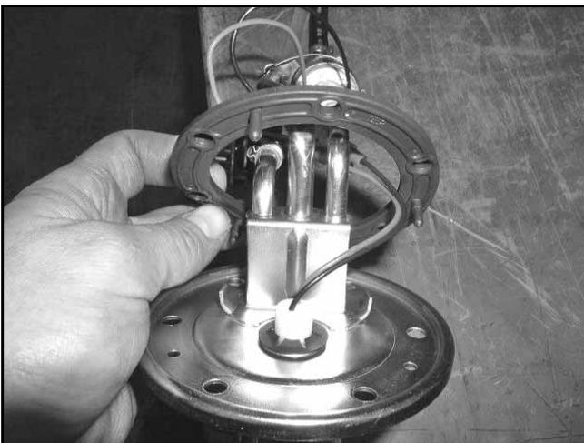
15. Carefully slide the pump assembly into the fuel tank until the gasket rests on the tank.
