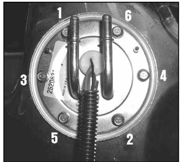
21. After installing the fuel pump assembly, the fuel tank must be tested for leaks by pressurizing the tank. See "Fuel Tank Pressure Test" on page 4.30.
