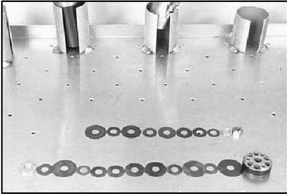
13. Inspect the valves for kinks, waves, pits or foreign material.
