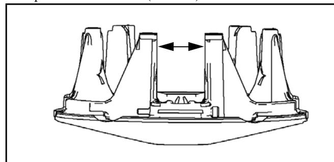
12. Subtract the spider measurement from the tower measurement. The clearance between the spider buttons and the moveable sheave towers is .002" - .004" (.05 - .10mm).
