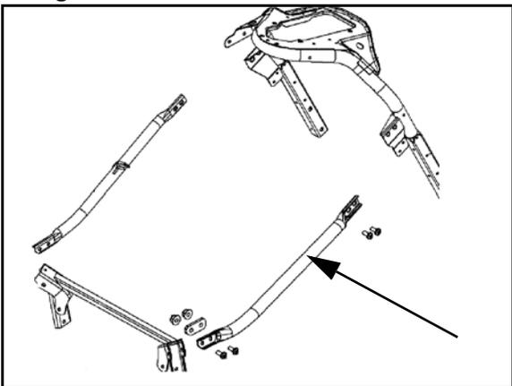
42. Replace the nosepan plugs were removed to access the front chassis brace fasteners.
