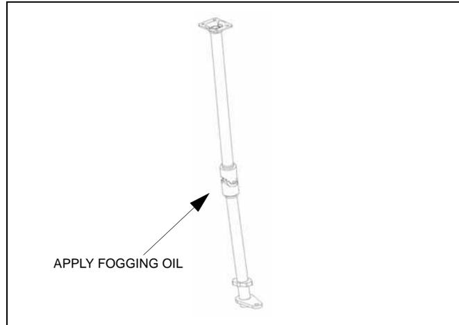
The rider select steering U-joint should be lubricated with Polaris fogging oil (PN 2870791).
