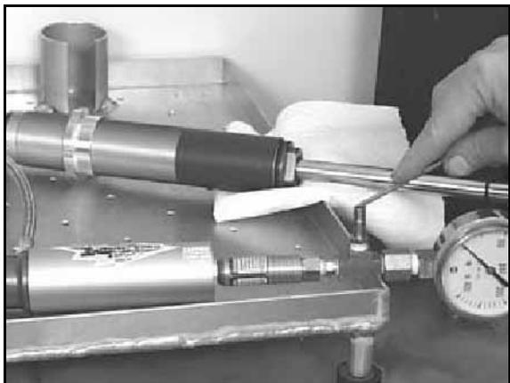
4. Press the end cap into the reservoir to access the snap ring.
