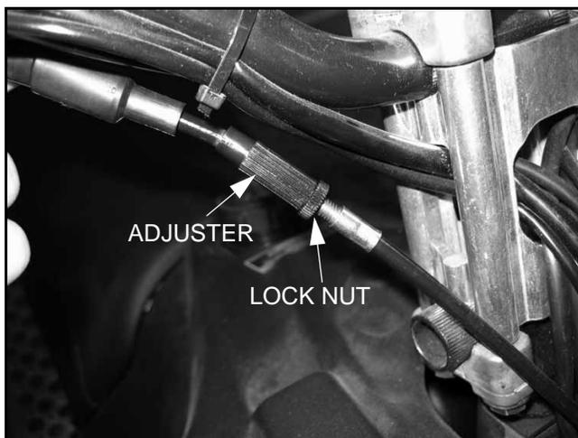
**NOTE: Never use the in-line adjuster to adjust engine idle speed and never adjust the cable so that the throttle plate cam on the throttle body no longer rests against the idle air gap screw.**
