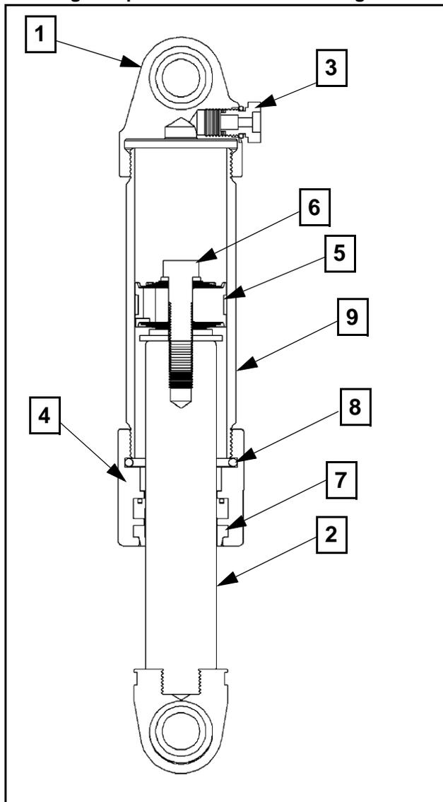
1. Place the body cap (1) of the shock in the vise so that the shock rod (2) is facing downward.
