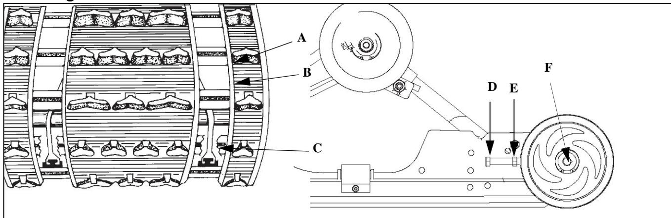
**NOTE:** *Track alignment affects track tension. Misalignment of the track will cause excessive wear to the track, rail slides, and rail.*
