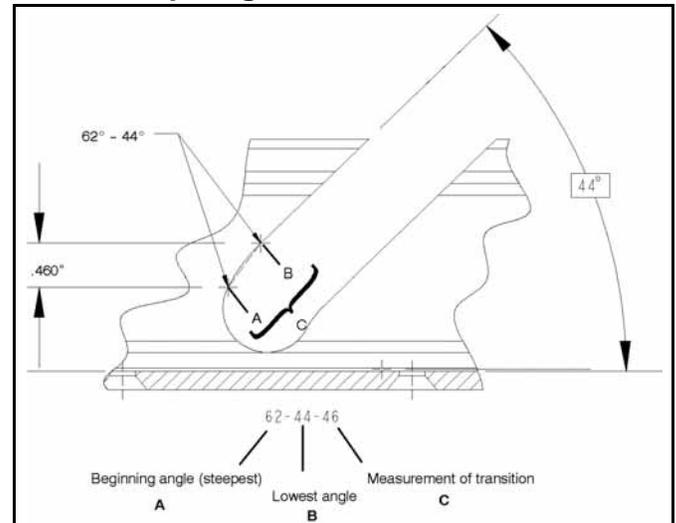
The angles and length of the transition between the first and final angle is stamped on the back of the helix. The first number (A) designates the starting angle of the ramp. The second number (B) designates the finish angle. The last number (C) is the transition distance (in inches) between the starting and finish angles.
