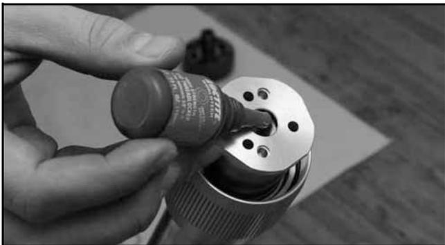
6. Torque bolt to specification.
