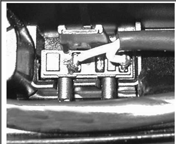
2. Unplug the brake light switch harness from the master cylinder.
