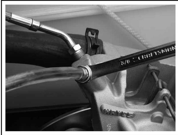
10. Torque the bleeder screw to 8-11 ft-lb (11-15 N-m).
