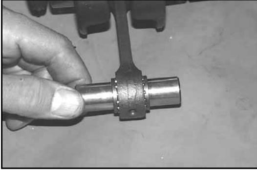
6. With pin and bearing centered in rod, twist ends back and forth in all directions to check for excessive axial play.
