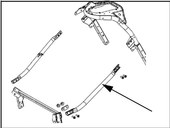
23. Apply Blue Loctite™ to the rear fasteners, install all the rear torque stop fasteners and torque to specification.
