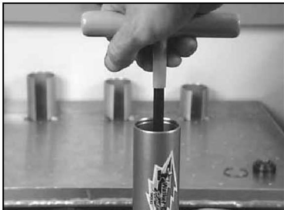
13. With the cylinder head assembly pushed down against the valve piston, dip the piston assembly in shock oil.
