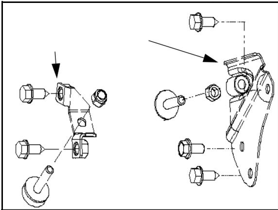
24. Remove the four engine mounting fasteners located on the engine straps.
