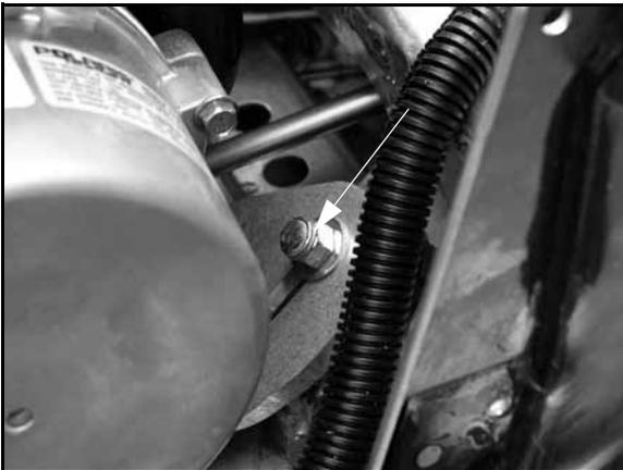
25. On CFI models, remove the Schrader valve cover located under the steering hoop, and depressurize the fuel rail. See "Fuel Rail Bleeding" on page 4.20.
