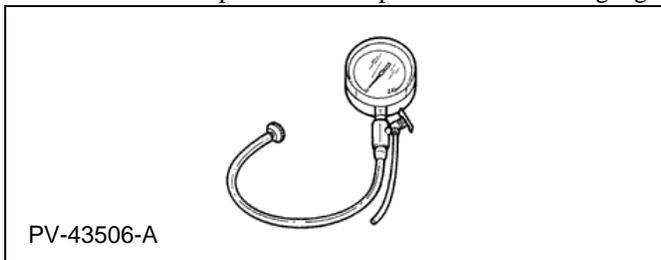
4. To observe running fuel system pressure, start the engine and compare reading to the specification.
