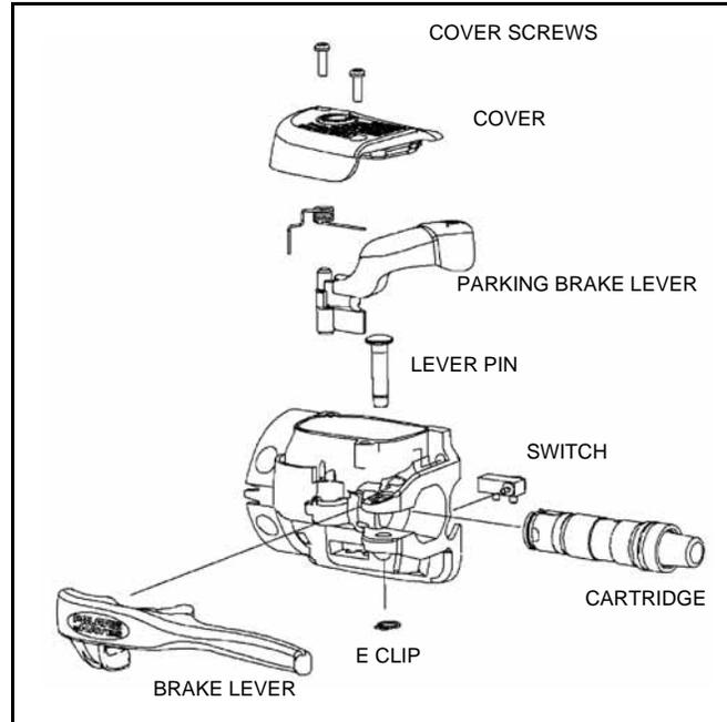
1. To remove the brake lever, remove the E clip from the lever pin.
