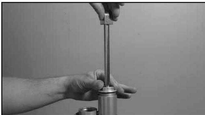
12. Using an adjustable wrench, secure the bearing cap assembly to the shock body.
