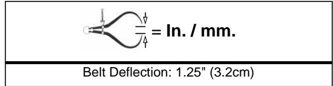
5. If the measurement is not correct adjust driven clutch.
