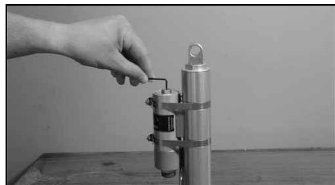
3. Slowly open the pressure valve assembly. Allow all of the nitrogen gas to escape from the reservoir and shock assembly.
