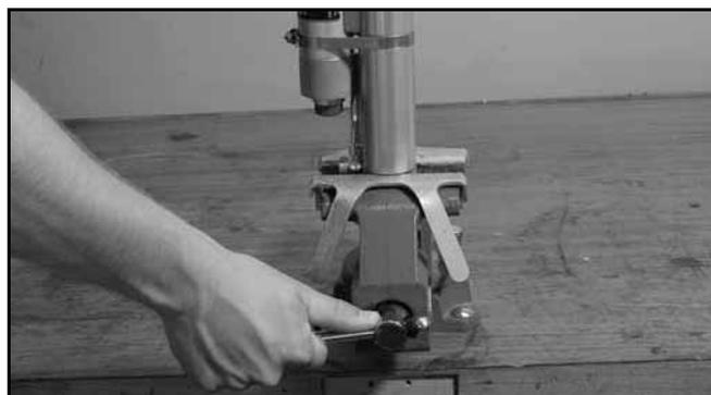
2. Remove the button head screw from the pressure valve assembly.
