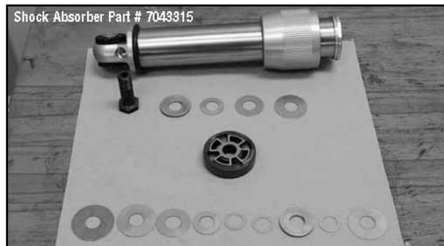
10. Remove the rod head assembly and spring from the rod shaft.
