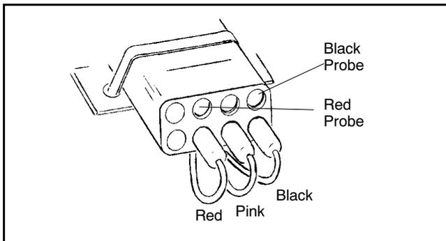
3. Connect the test tool to the TPS on the carburetor or throttle body.
