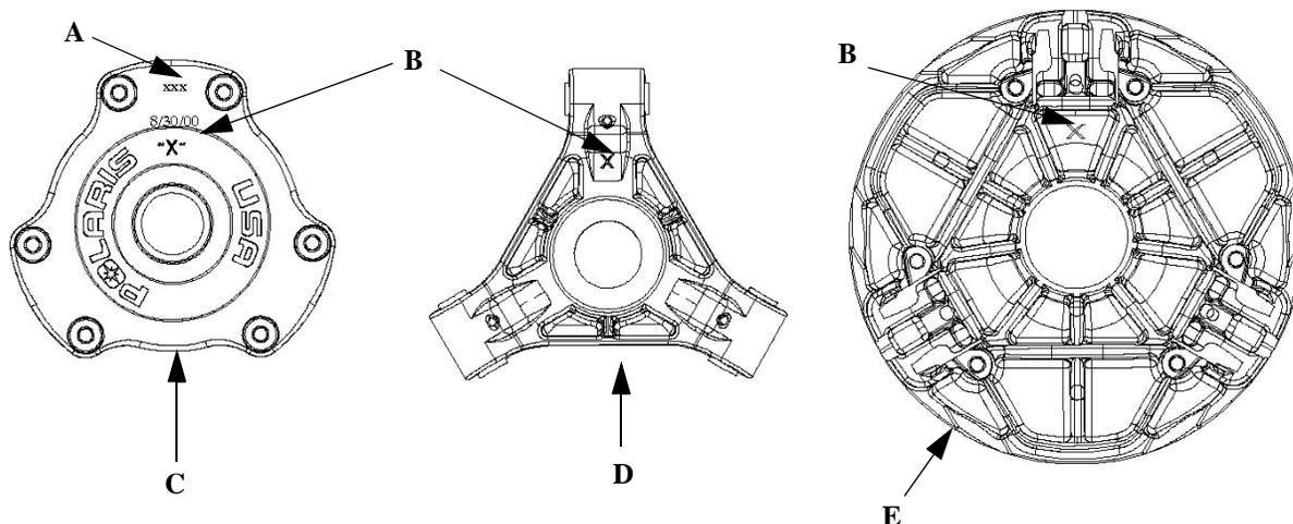
Every clutch will have the last three digits of the clutch part number etched on to the cover (A). The “X” (B) marking is an index mark where the clutch cover (C), clutch spider (D) and the stationary sheave (E) should line up when the clutch is assembled.
