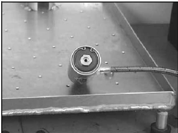
3. Insert safety needle carefully and depressurize the shock.
