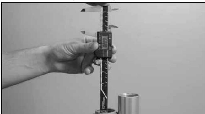
9. When the IFP is set to the depth specification, reinstall the bleed screw.
