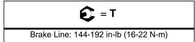
13. Tighten the brake line into the master cylinder in an orientation so that the line does not have any sharp bends when it is installed on the handlebar.
