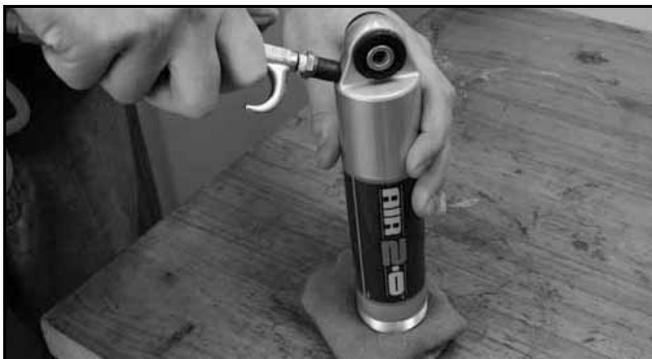
9. Place the 36mm piston (shock) rod upper mount in a soft-jawed bench vise. Remove the piston valve and valve shim assembly from the rod in the sequence of disassembly.
