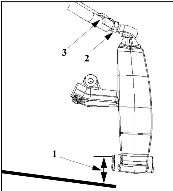
1. Raise the front of the machine so that the skis are off the floor 3" (7.62cm). The shocks should be at full extension
