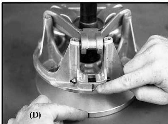
Vary the amount and thickness of spacer washers (washer thickness may vary slightly). Re-index marked spider leg to another tower. This can be done because spider has little effect on overall clutch balance.
