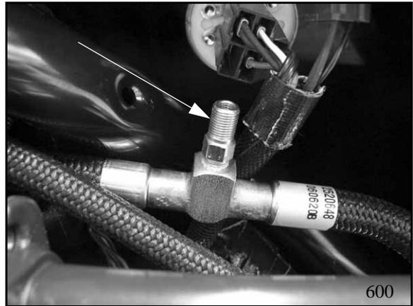
26. Using the fuel line disconnection tool (PN PS-47152) (20), separate the fuel filter and the fuel return line.
