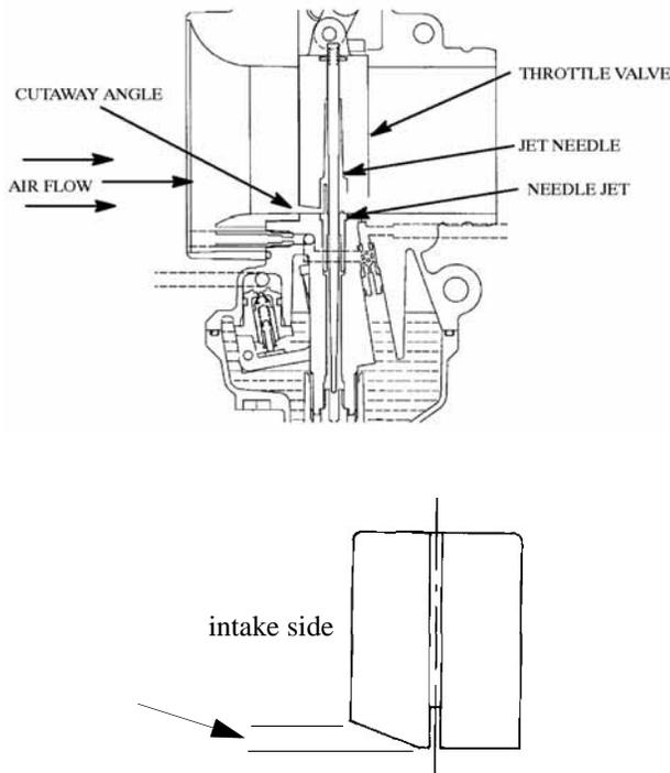
The throttle valve controls the rate of engine air intake by moving up and down inside the main bore. At small throttle openings, air flow control is performed chiefly by the cutaway. By controlling air flow the negative pressure over the needle valve is regulated, in turn varying the fuel flow.
