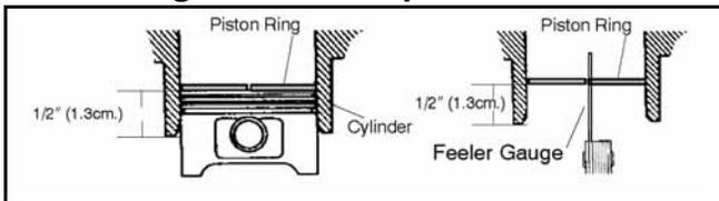
Position the ring 1/2" (1.3 cm) from the top of the cylinder using the piston to push it squarely into place. Measure installed gap with a feeler gauge at both the top and bottom of the cylinder.
