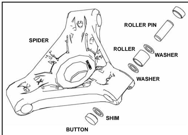
1. With the spider in a vise start removing the spider buttons by drilling a 0.18" hole in the center of a button on one side of the spider.
