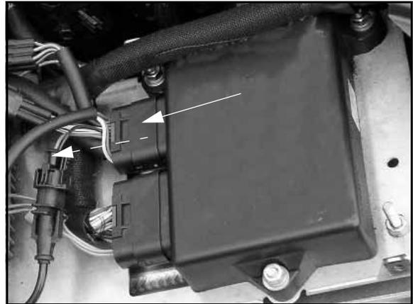
11. Disconnect the regulator/rectifier connections.
