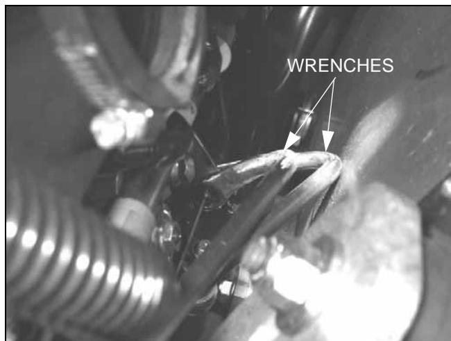
11. When adjusting the lever, make adjustments in small increments, then re-check the timing mark alignment.
