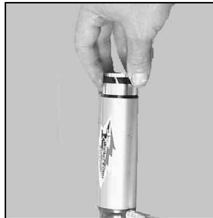
10. Screw the IFP tool, PN PS-45908, into the IFP.
