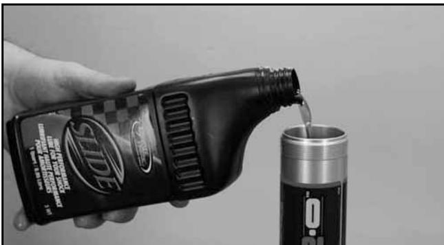
**NOTE:** Allow the shock to stabilize for several minutes and allow the air bubbles to escape to the top.
