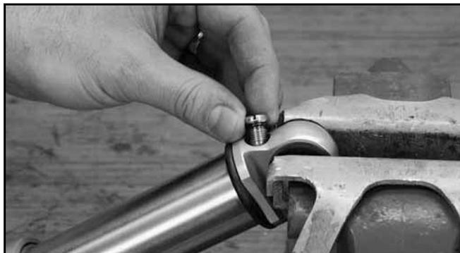
6. Using interlocking channel pliers, loosen and remove the cylinder head assembly.
