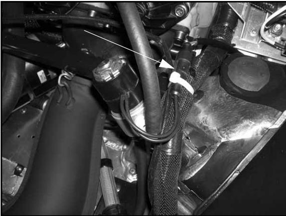
14. Disconnect the EV vent lines from the EV base and secure the vent lines out of the way.
