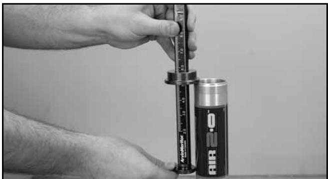
12. Apply a thin layer of oil to the IFP, wearband, and o-ring. Insert the IFP, o-ring side first, into the shock body.
