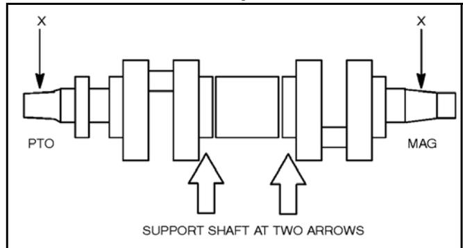
1. Support the crankshaft in a set of "V" blocks as shown.
