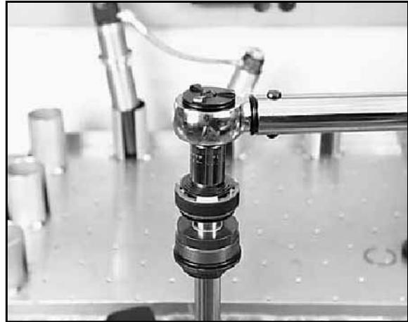
5. Secure the shock body by its lower mount.
