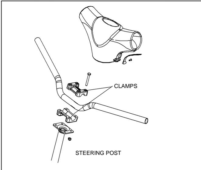
1. To adjust the handlebar angle, remove the handlebar cover to expose the clamp.
