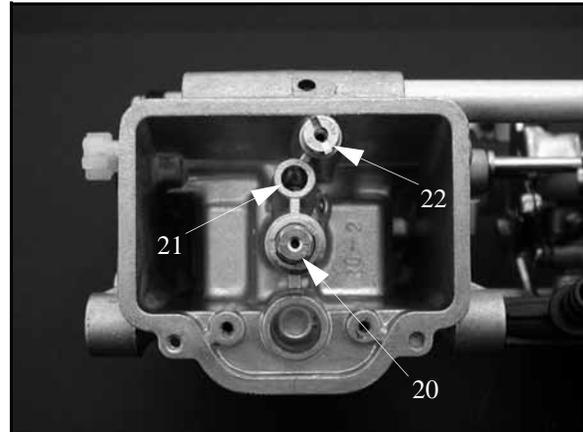
16. Clean out all passages in carburetor body with carburetor cleaner. Dry all passages and jets with compressed air.
