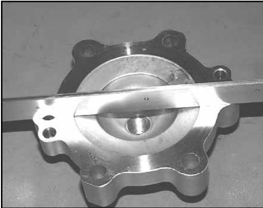
Using a flat bar and a feeler gauge, inspect each cylinder head for warping. Replace head if warping exceeds .003" (.08mm).
