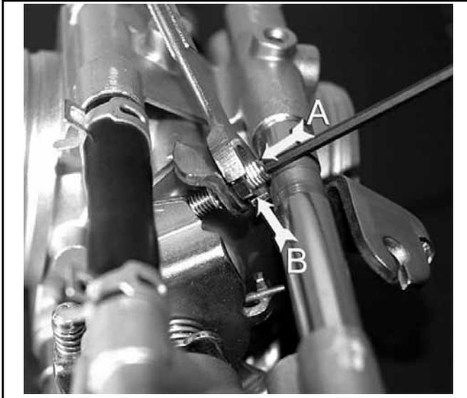
4. Reinstall the throttle cable, then install the throttle body back on to the engine.
