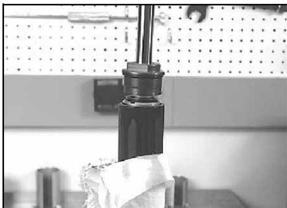
14. Fill the shock body with oil to the bottom of the threads. Carefully insert the piston rod and valve assembly into the cylinder.
