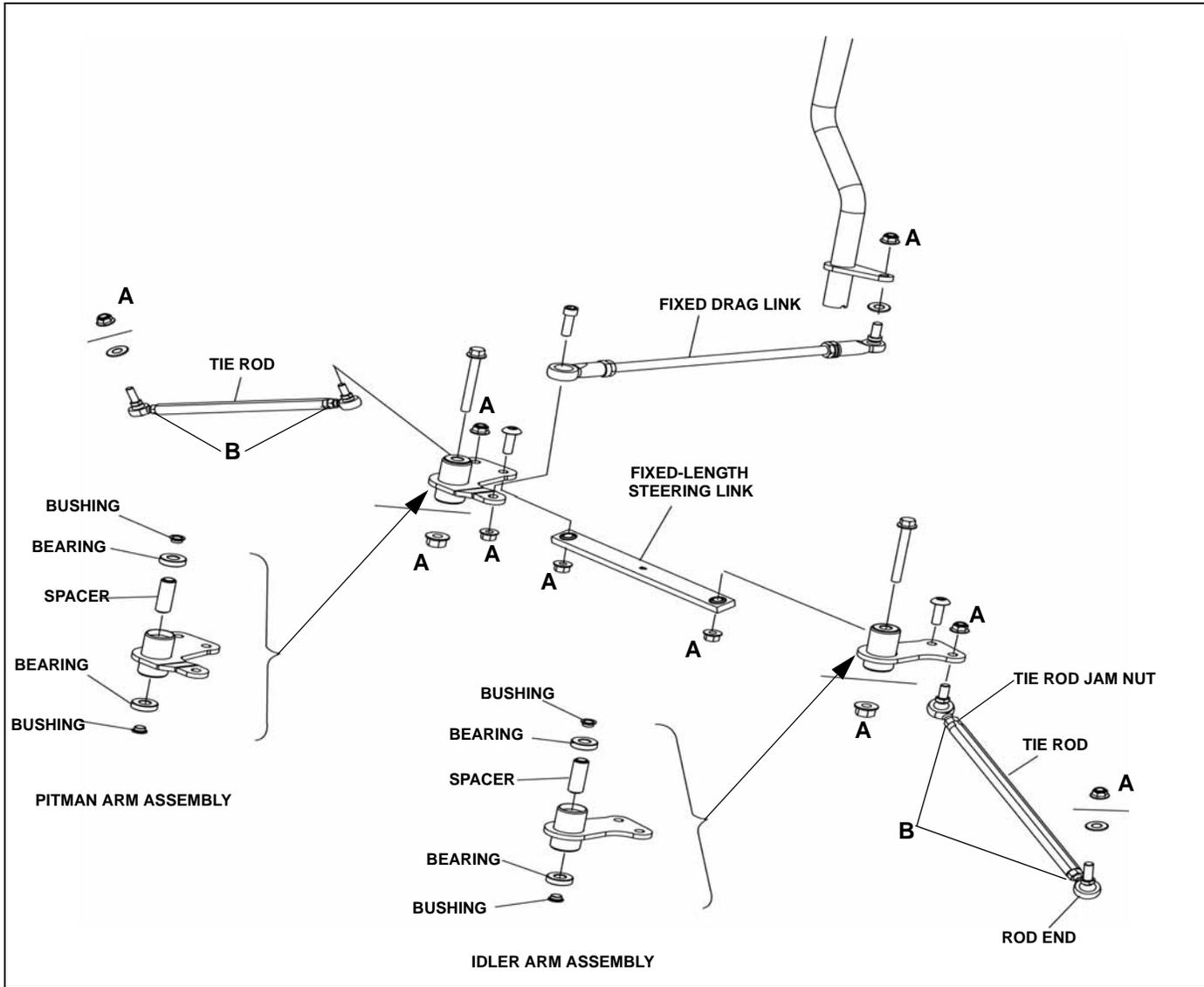
**NOTE:** 2008 IQ steering linkage shown. 2007 models feature adjustable steering links.
