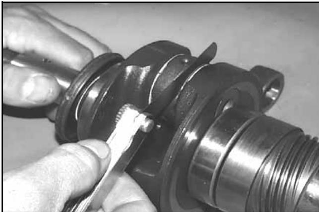
Measure connecting rod big end side clearance with a feeler gauge on both sides of the connecting rod. The side clearance on either side of the connecting rod cannot exceed the connecting rod side clearance specification. The difference between the two clearance measurements
