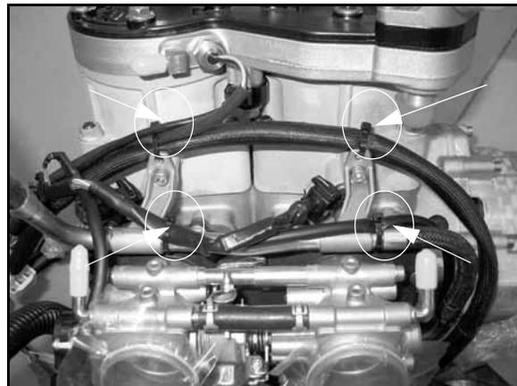
**NOTE: The engine must be removed from the engine compartment to access the lower two fuel injectors.**
