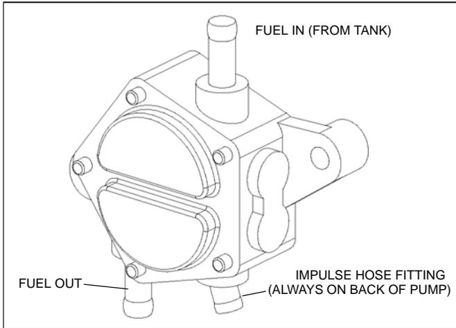
The impulse-powered fuel pump on carbureted engines works by using the positive and negative pressure pulses generated by the movement of the pistons inside the engine crankcase.
