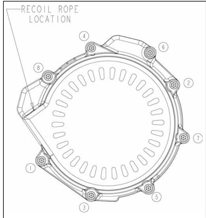
Carbureted Crankcase Torque Pattern
