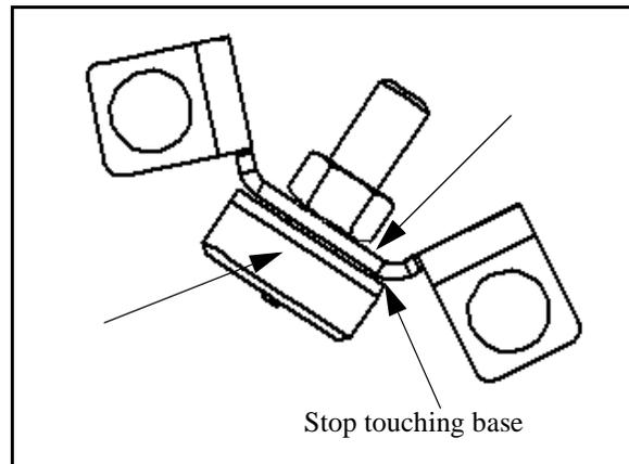
26. Install the front torque stop assembly and torque the plate fasteners to specification.
