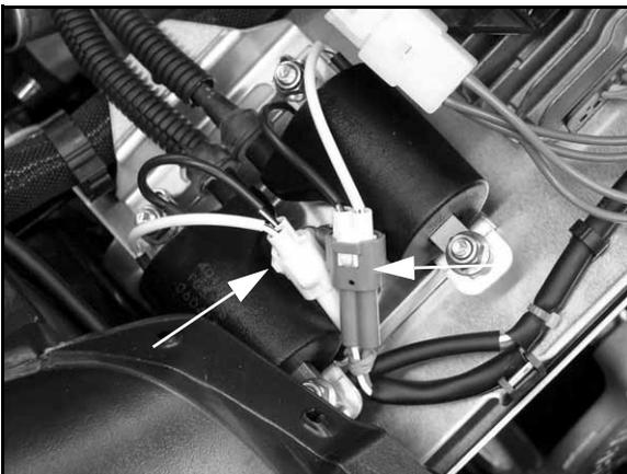
37. Connect the regulator rectifier connections.
