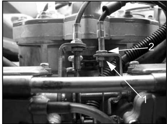
3. Turn sleeve adjusting nut (2) counter-clockwise until the choke toggle shows no free play when pulled, then rotate it clockwise until there is between 1/8 - 1/4in (3.2-.6.4mm) free play (3).
