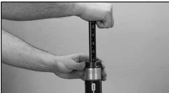
14. Install the pressure valve assembly into the valve port and torque to specification.
