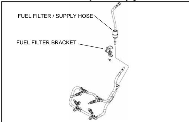
2. After de-pressurizing the fuel system and disconnecting the fuel hoses, remove the fuel filter cartridge from the bracket. Dispose of any fuel in an appropriate container, then discard assembly.
