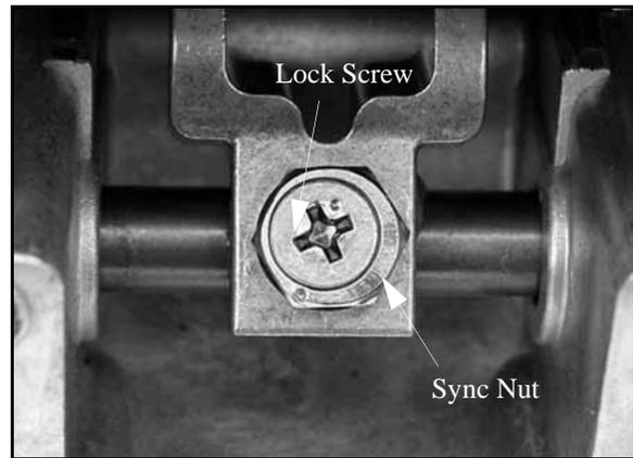
8. Adjust the synchronization nut until it is even with the PTO slide.
