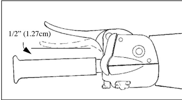
The gap between the brake lever and handlebar grip should be equal to or more than 1/2" (1.27cm) when depressing the brake lever.
