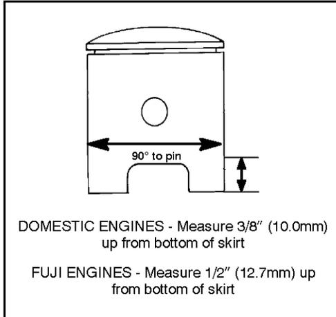
Subtract this measurement from the minimum cylinder measurement (90° to the pin). If clearance exceeds the service limit, the cylinder should be re-bored (replaced if Nicasil-lined) and new pistons and rings installed.
