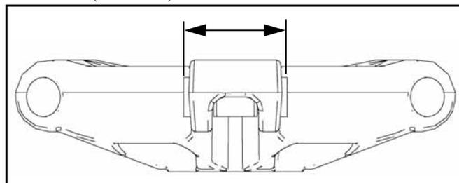
11. Measure the width of the moveable sheave towers. Specification is 1.50" (38.1mm).
