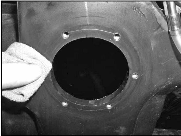
14. Install a new, clean gasket by carefully sliding it over the fuel lines, and pump components. Position the gasket with the barbs/locating pins facing the flange. Align the pins/barbs with the holes, then push and pull the barbs/pins through the holes in the flange.
